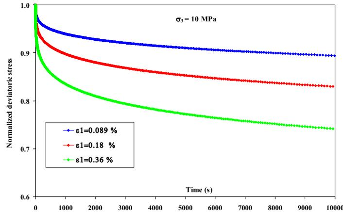
Fig. 6. Simulation of relaxation test per stage ( $\sigma_3 = 10$  MPa) at three levels of deviatoric stress ( $q = \sigma_1 - \sigma_3$ ):  $q = 5$  MPa ( $\varepsilon_1 = 0.089\%$ ),  $q = 10$  MPa ( $\varepsilon_1 = 0.18\%$ ) et  $q = 25$  MPa ( $\varepsilon_1 = 0.36\%$ )
