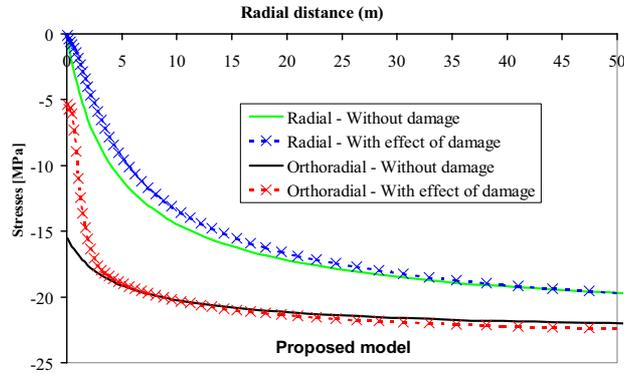
Fig. 9. Comparison of radial and orthoradial stresses at steady-state: continue ( $A_0=1.9e-2 \text{ h}^{-1}$ ;  $n=3$ ;  $m_0=m_1=-1e-20$ ;  $b_1=0$ ); cross ( $A_0=1.9e-2 \text{ h}^{-1}$ ;  $n=3$ ;  $m_0=m_1=-1e-20$ ;  $b_1=1.6$ )
