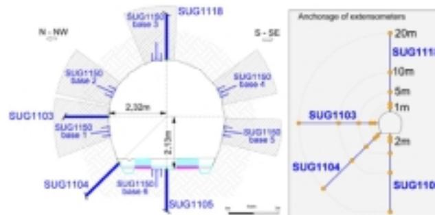
Fig. 1. Convergence measurements and extensometers in section SMR1.1
