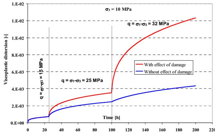
Fig. 7. Viscoplastic shear strain for a multi-stage creep test simulation (1<sup>st</sup> stage  $q = 15$  MPa; 2<sup>nd</sup> stage  $q = 25$  MPa and 3<sup>rd</sup> stage  $q = 32$  MPa)
