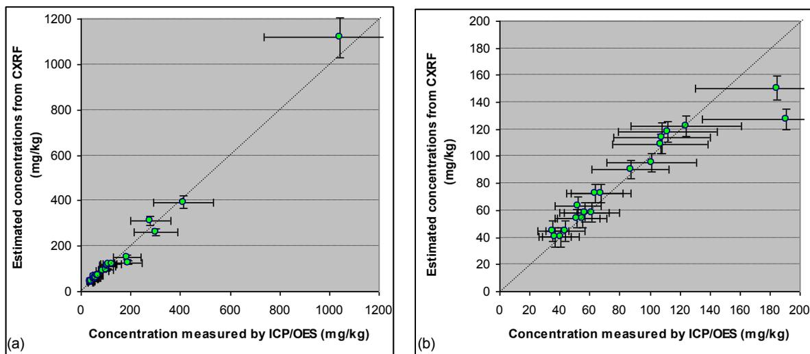
Figure 2 : Comparison of the lead concentration measured by ICP/OES with the predicted concentrations based on equation 1 - (a) : a view of the whole range of concentrations tested, (b) : an enlargement for concentrations inferior to 200 mg/kg
