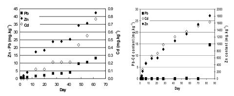
At the end of experiment, the amount of elements released was very low in comparison with the initial content of mining wastes Figure 3. It reached 0.2% for Zn and for Pb and 1.4% for Cd, 3.6 % for  $SO_4^{2-}$  and 2.5 % for Ca. The metals amount released into solution were very small reflecting a retention mechanism of Pb, Zn and Cd in the mining wastes.
