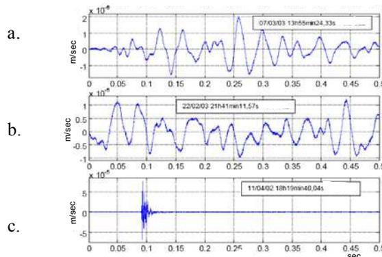
Figure 2: Example of seismic events recorded during the cavity flooding : a) seismic event associated with mining blasting; b) seismic event associated with natural earthquake; c) local seismic event induced by the cavity flooding. The example shows signals recorded by the vertical sensor GL.
