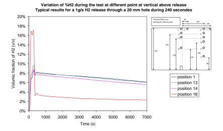
Figure 10 : variation of % H<sub>2</sub> for a 1 g/s H<sub>2</sub> release through a 20 mm hole
