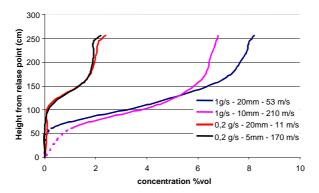
Figure 12 : concentration profile (along a vertical located at x = 1.40 m and y = 0 m) for various releases after release phase
