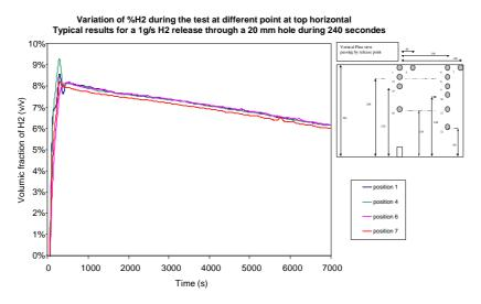
Figure 9: variation of % H<sub>2</sub> for a 1 g/s H<sub>2</sub> release through a 20 mm hole
