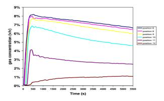
Figure 17: variation of %H2 for 1 g/s H<sub>2</sub> release through a 20 mm hole
