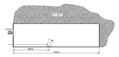
Figure 4: Injector location in the y-direction
