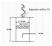
Figure 5: Hydrogen injector
