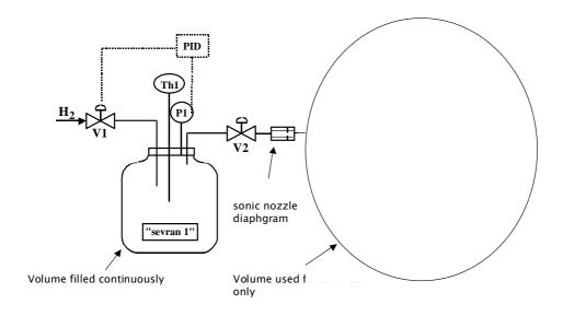
Figure 6: mass flow rate measurement
