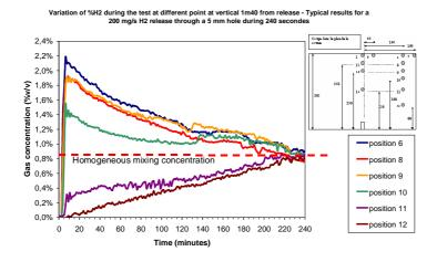
Figure 11: variation of %H<sub>2</sub> for 0.2 g/s H<sub>2</sub> through a 5 mm hole
