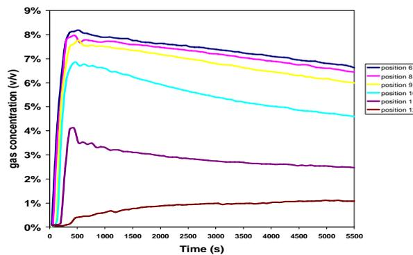
Figure 17 : variation of %H<sub>2</sub> for 1 g/s H<sub>2</sub> release through a 20 mm hole
