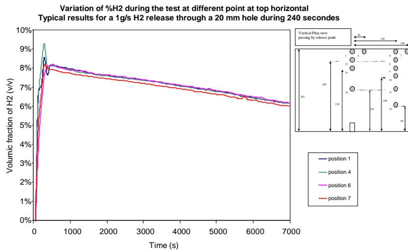
Figure 9 : variation of % H<sub>2</sub> for a 1 g/s H<sub>2</sub> release through a 20 mm hole
