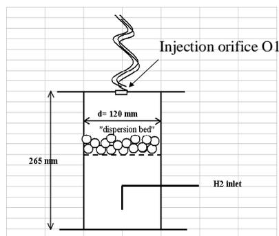
Figure 5 : Hydrogen injector
