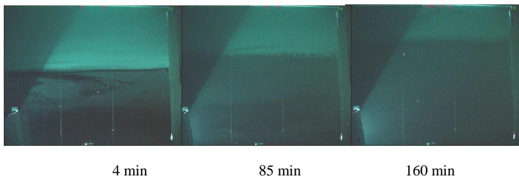
Figure 15 : view of helium release for a 1,84 g/s flow rate through a 20 mm hole during the diffusive phase
