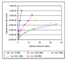
Figure 4. Injection flow rate/injection pressure.
