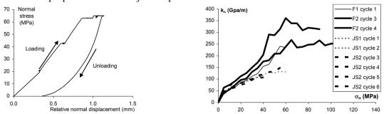
Figure 3.  $\sigma_n$  against  $u_n$  for F1 sample (left) and  $k_n$  against  $\sigma_n$  for all samples (right).
