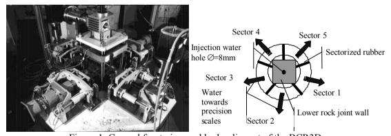
Figure 1. General front view and hydraulic part of the BCR3D.
