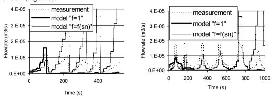
Figure 9. Comparison between measured and computed injection flow F1 (left) and JS1 (right).
