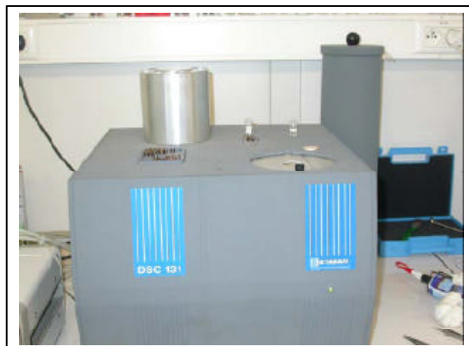
Illustration 1: DSC Calorimeter used for tests
