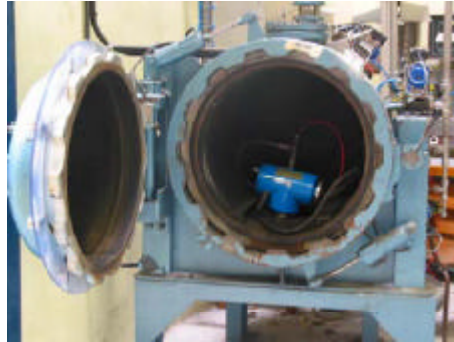
Figure 3: Front view of a typical test chamber to test ignition potential of equipment
