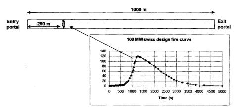
Fig.8: fire scenario of the basic example
