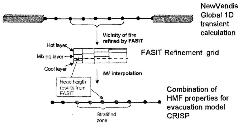
Fig. 5: coupling schematic of smoke dispersion models
