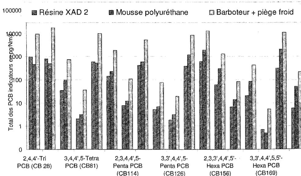
From this figure, it is clear that the washing bottles are far more efficient than the two solid adsorbents, even for light PCBs. The efficiency of washing bottles with hexane is 10 times higher than the PUF one and 20 times higher than the XAD 2 one.
