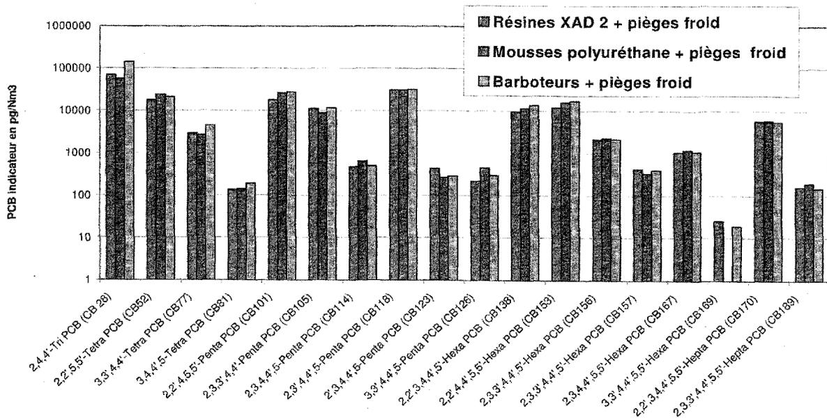
By using two sampling devices and two cold traps together, results are very similar for each of the 3 methods and for each of the 18 PCBs. The only exception being the lighter tri PCB where the concentration obtained by the washing bottle method is twice the values obtained by the 2 other methods.
