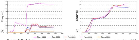
Figure 17: Evolution or total ansupated work in plastic deformation (a) and total orlergy released (b)
