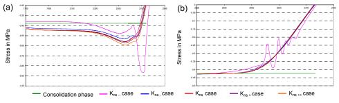
Figure 6: Horizontal (a) and vertical (b) stress profiles at a depth of 16 m (in JCB limestone)
