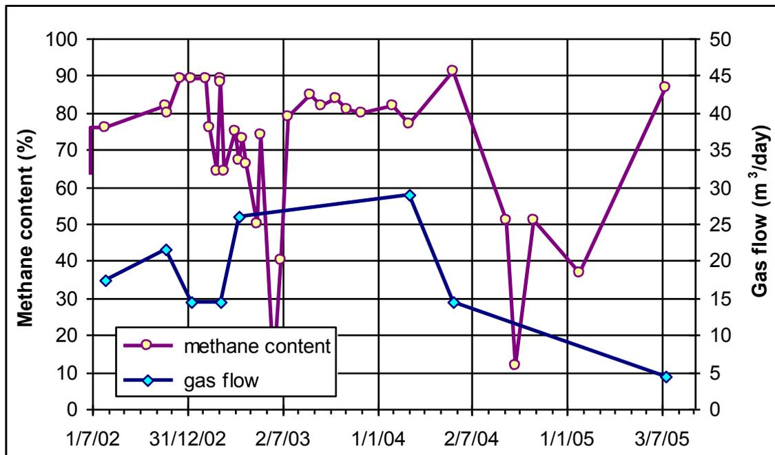
Figure 8. Example of the activity of a decompression borehole in the Decazeville coalfield
