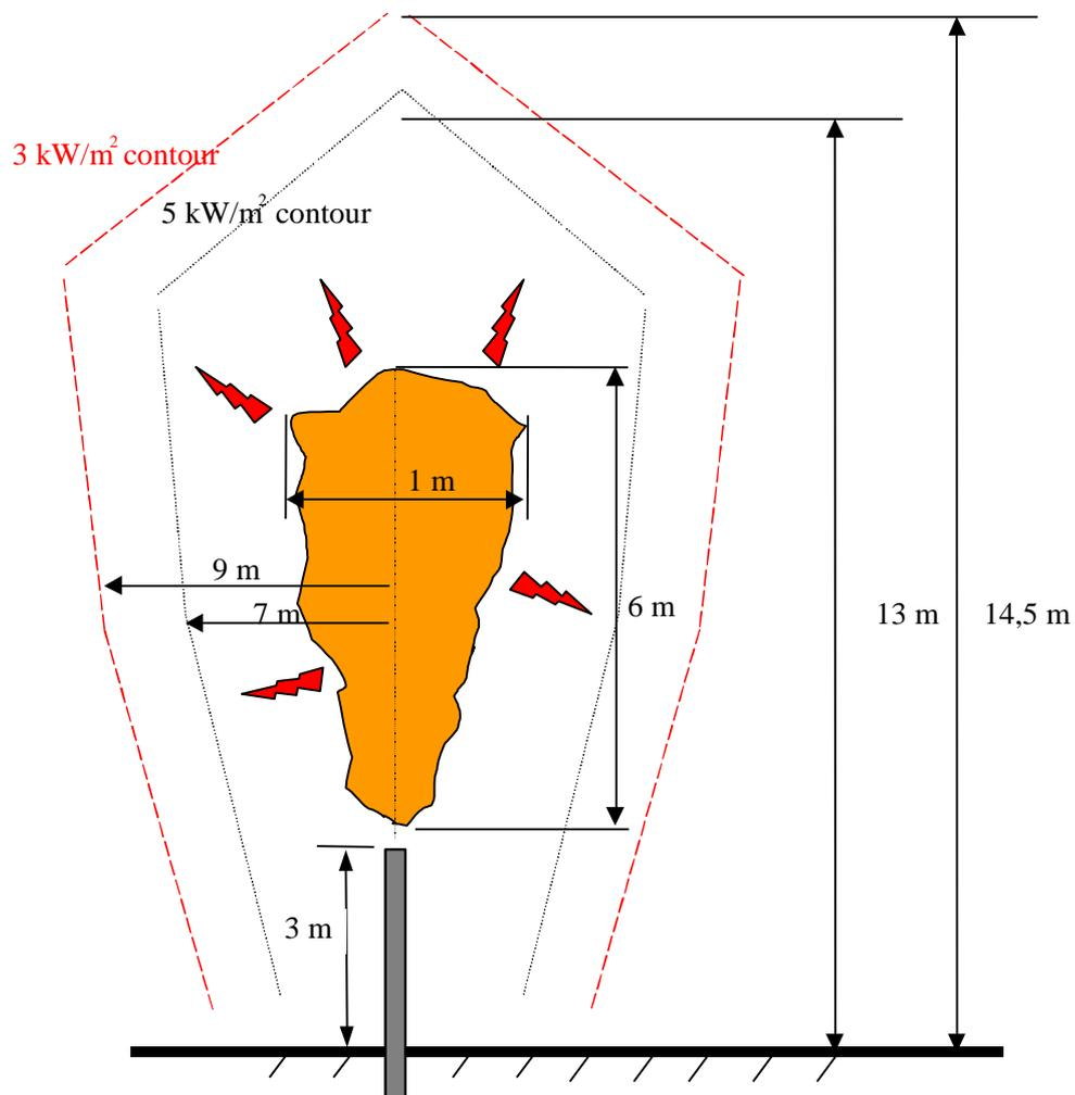
Figure 7. Example of the definition of the protection area around a highly active decompression drilling in relation to the thermal effects linked to accidental gas inflammation (methane outflow  $0,3 \text{ m}^3/\text{s}$ )
