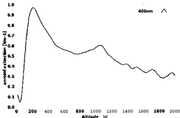
Figure 4: Typical Lidar signal at 400nm during POVA campaign.
