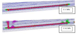
Figure 4: Simulation of the behaviour of shallow workings for c = 1 MPa and c = 0.5 MPa
