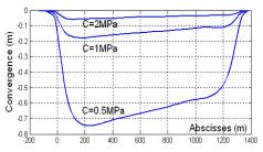
Figure 3: Evolution of pillar convergence in a panel as a function of coal cohesion values.
