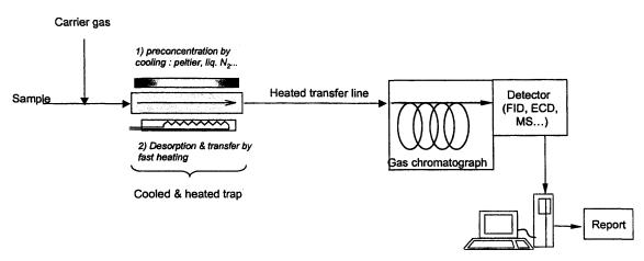
Figure 1 : general principle of preconcentration & analysis.
