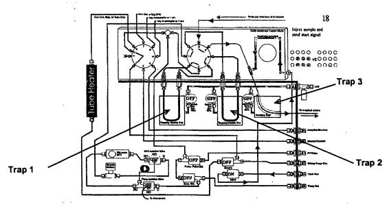
Figure 3 : pneumatics of Entech preconcentrator
