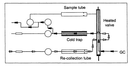
Figure 4 : SecureTD<sup>™</sup>: re-collection of the split part of the sample (Markes International Ltd)
