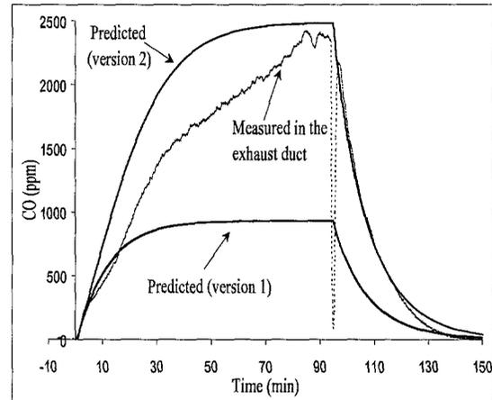
Figure 7. Comparison of measured and predicted CO concentrations (ventilation rate =280 Nm<sup>3</sup>.h<sup>-1</sup>)
