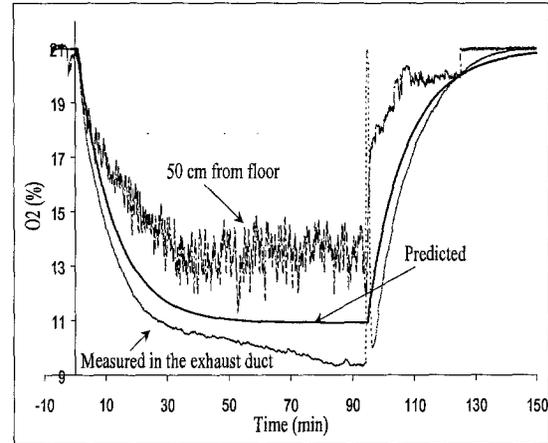
Figure 5 . Comparison of measured and predicted O<sub>2</sub> concentrations (ventilation rate =280 Nm<sup>3</sup>.h<sup>-1</sup>)
