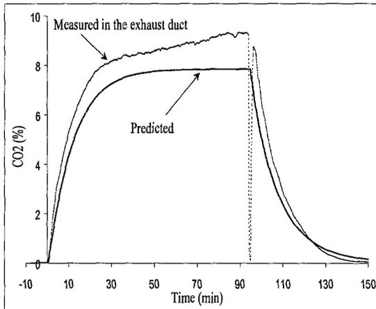
Figure 6. Comparison of measured and predicted CO<sub>2</sub> concentrations (ventilation rate =280 Nm<sup>3</sup>.h<sup>-1</sup>)
