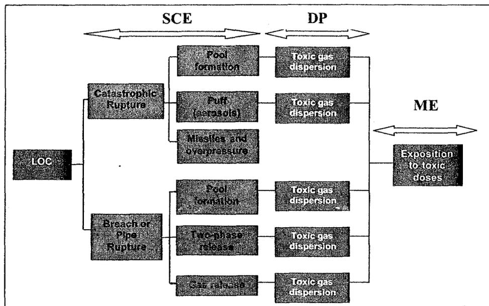
Figure 3 : MPPS for a pressurised vessel of chlorine
