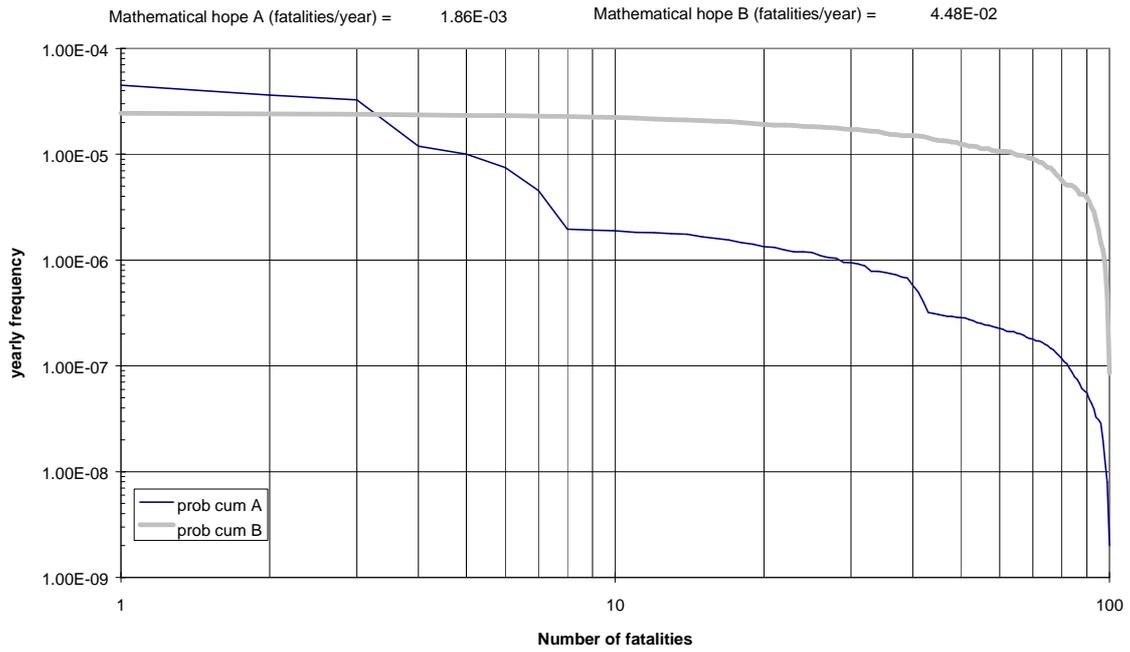
**Figure 3 : Comparison of a F/N curve with an acceptance criteria**
