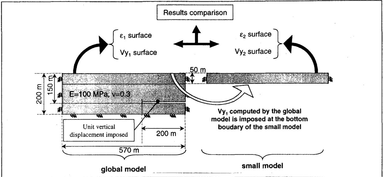
Figure 5 : Comparison between global and small models.
