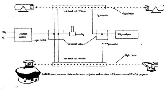
Figure 2 : test-bench for SO<sub>2</sub> set up in tunnel
