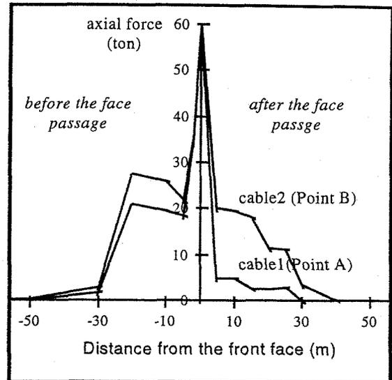
Fig. 12 : Evolution of cable axial strength
