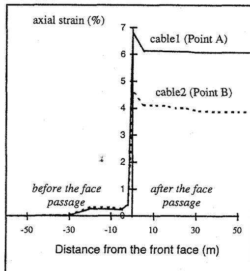
Fig. 13 : Evolution of cable axial strain
