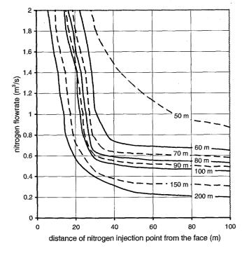
Figure 5. Optimization of Nitrogen Injection (Each Line Shows the Position of the 1 % O2 Fringe in the Goaf for Given Flowrates and Locations of Injection; Figures Indicate the Distance of this Fringe From the Face Line)
