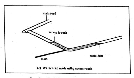
Figure 3: Rapid closure of a district by water trap
