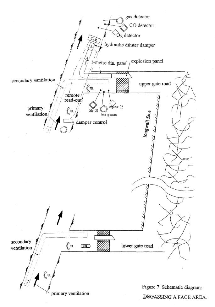
Figure 7: Schematic diagram: degassing a face area.
