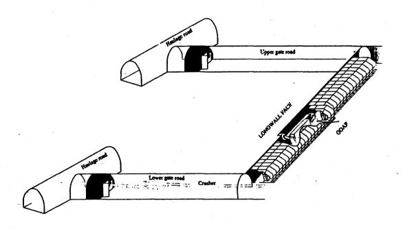
Figure 2: Diagram of a mechanised retreating longwall face
