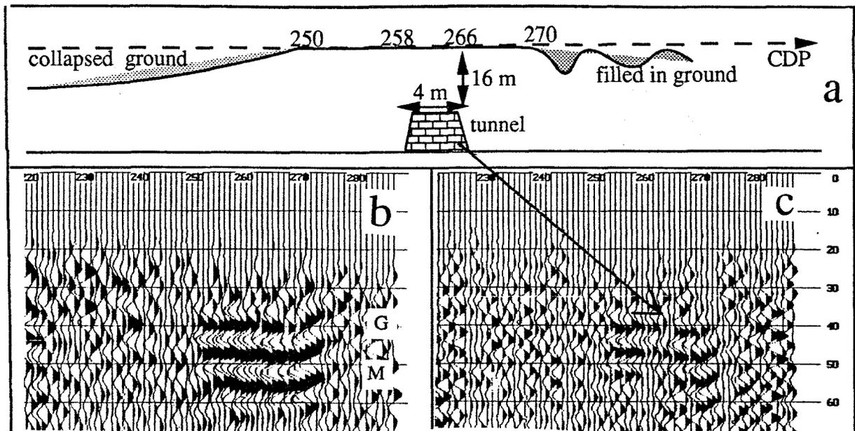
Fig.3: (a) Position of the profile S2 in regard to the location of the tunnel and of the collapsed zone; (b) obtained seismic section for  $D/\lambda=0.65$  and  $S_c/S_f=0.3$ ; (c) Same as (b) except for  $D/\lambda=0.9$  and  $S_c/S_f=0.43$
