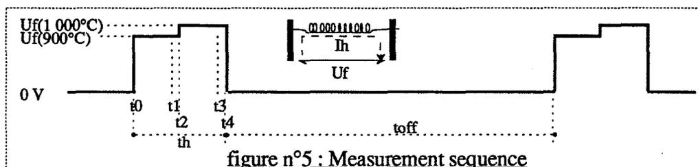
$t_0$ : filament heated to  $900^\circ\text{C}$
