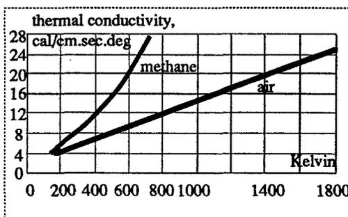
figure n°11 : thermal conductivity
