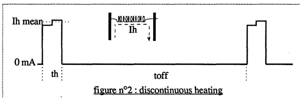
$$I_{\text{mean}} = I_{h\text{ mean}} \times \frac{t_h}{t_h + t_{\text{off}}} \quad [2]$$
