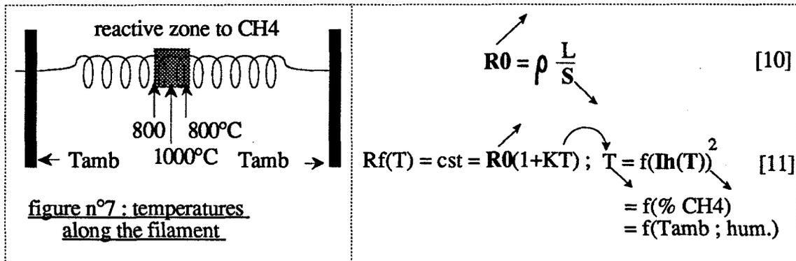
$R_0$  thus increases with wear [10], with the result - owing to the principle of constant resistance heating - that there is a negative drift in the heating currents and in the response at 900°C and 1000°C [11].
