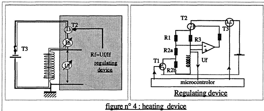
The response of the filament also results in a change in  $U_f$  which follows the change  $I_h$ . In fact  $U_f = R_f \times I_h$  where  $R_f$  is constant by definition.
