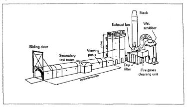
Figure 3: INERIS fire test gallery
