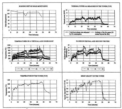
Figure 4: Main characteristics recorded during the 1 m² heptane test in the INERIS fire gallery (S1: cross section located 2.5 m downwind from the fire; S2: 5 m, S3: 10 m; S4: 20 m; S5: 40 m)
