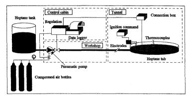
Figure 2: Experimental installation for heptane tub fires
