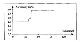
Figure 14: Ventilation conditions for heptane test H32
