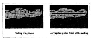
Figure 7: Influence of ceiling configuration on backlayering limits
