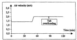
Figure 10: Ventilation conditions for heptane test H21
