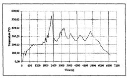
Figure 8: Temperature at the ceiling, above the fire
