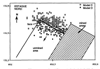
Fig.9: Location of 200 tremors compared: model B locates the cloud at the back of the face and model (new multilayered model) locates the cloud at the level of, and in front of the face.
