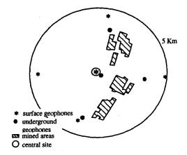
Figure 1: geometry of the seismic array with mined layout mapped
