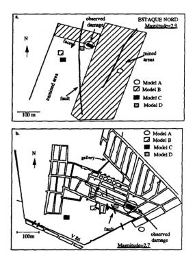
Fig. 8: Comparison of rockbursts located with velocity models A, B, C and the new velocity model D.
