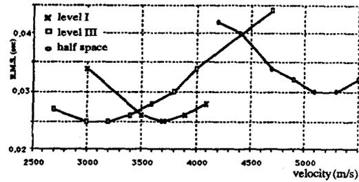
Fig.7 : Analysis of the average R.M.S. as a function of the propagation velocity from a population of 188 microseismic events.
