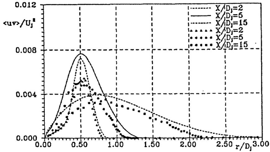
Fig. 9 : Radial distributions of the Reynolds stress for Air-Air jet.
