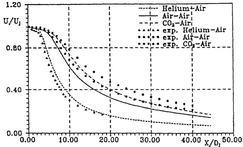
Fig. 5 : Evolutions of the velocity half-width on the jet centerline.
