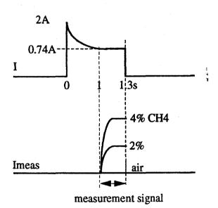
Characteristics of the GTM741 mine gas detector using this technique:
