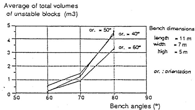
Fig. 6 : Optimisation of orientation and bench angles.
