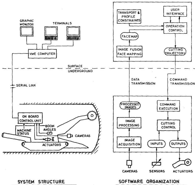
Figure 7. Control system structure
