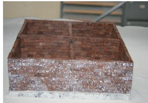
Figure 3. Physical model of masonry structure using wood pieces
