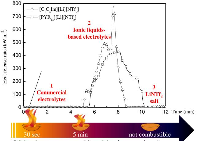
Major improvement achieved by increased resistance to ignition when replacing carbonates by ionic liquids as electrolyte solvents
