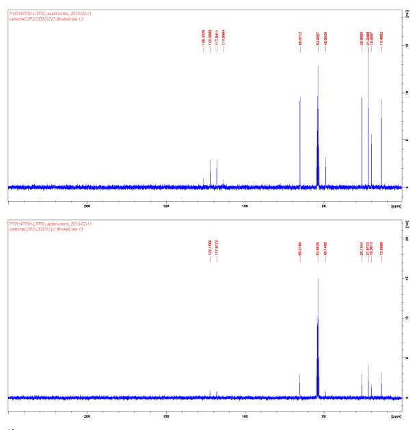
$^{13}$ C NMR spectra of [PYR<sub>14</sub>][Li][NTf<sub>2</sub>] before (top) and after (bottom) thermal treatment
