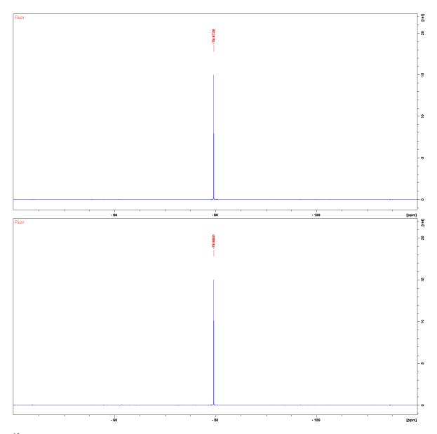
$^{19}\mathrm{F}$  NMR spectra of  $[C_1C_4\mathrm{Im}][\mathrm{Li}][\mathrm{NT}f_2]$  before (top) and after (bottom) thermal treatment
