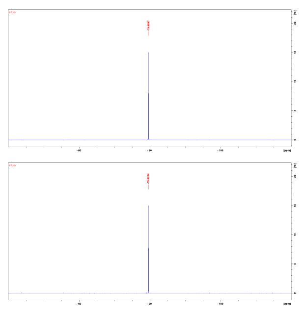
$^{19}$ F NMR spectra of [C<sub>1</sub>C<sub>4</sub>Im][Li][NTf<sub>2</sub>] before (top) and after (bottom) thermal treatment
