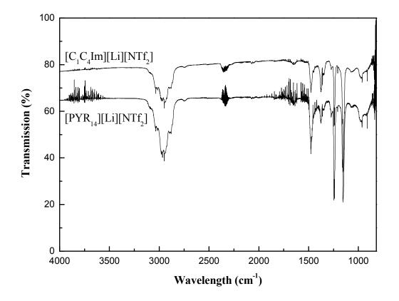
SI-6: Infrared spectra of electrolytes gas phase (after blank subtraction)
