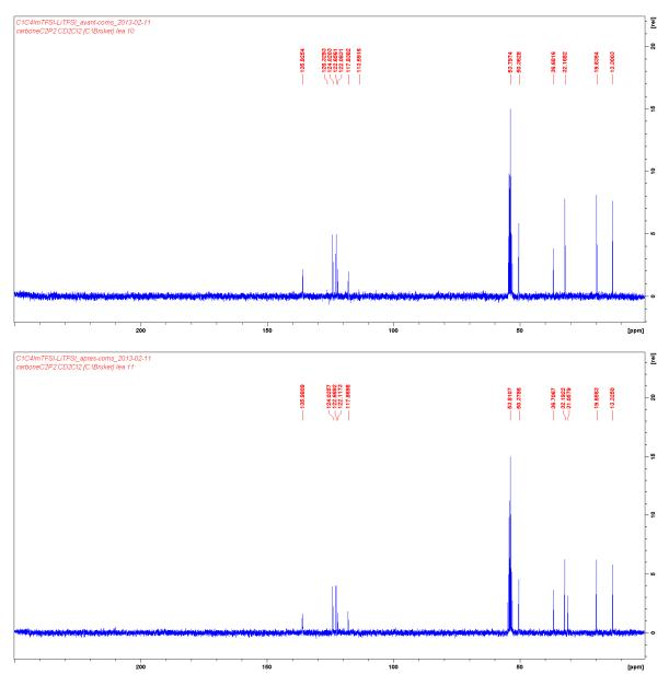
$^{13}C$  NMR spectra of  $[C_1C_4Im][Li][NTf_2]$  before (top) and after (bottom) thermal treatment
