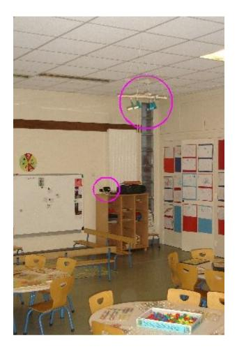
Figure 1. Passive samplers of formaldehyde and benzene near the ceiling, and the Lum'air sensor
