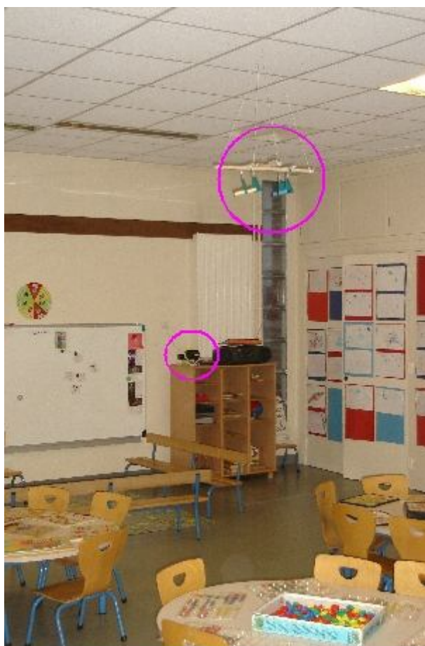
Figure 1. Passive samplers of formaldehyde and benzene near the ceiling, and the Lum'air sensor at the back of the room (source: Air Normand).
