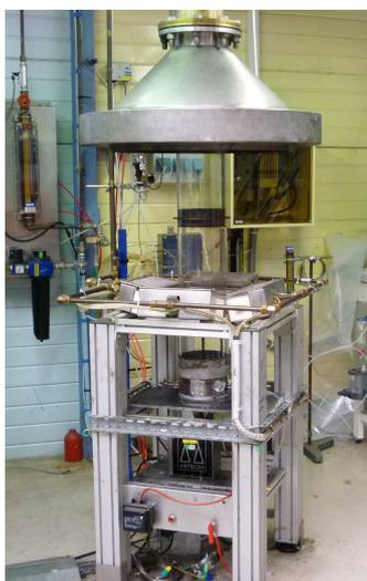
**Figure 1.** The Fire Propagation Apparatus
