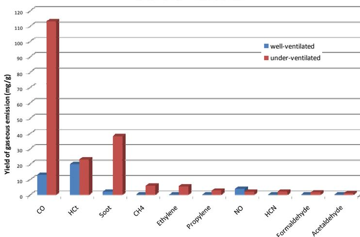
**Figure 11.** Emission yields of various gases from combustion of PMMA - 5Al<sub>2</sub>O<sub>3</sub> - 10 APP in controlled-ventilation conditions
