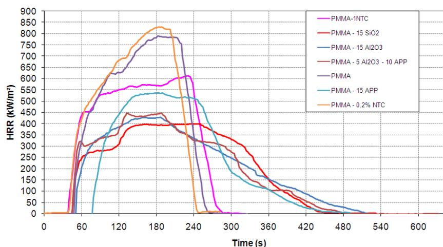
**Figure 2.** Heat Release Rate measuring during tests in well-ventilated conditions
