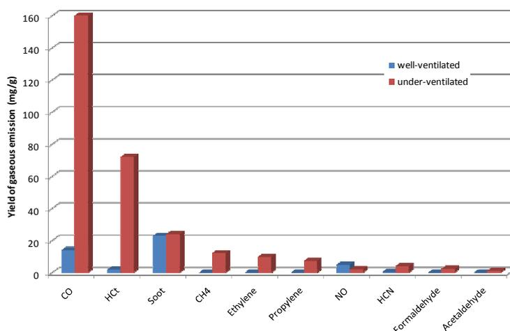
**Figure 10.** Emission yields of various gases from combustion of PMMA-15 APP in controlled-ventilation conditions
