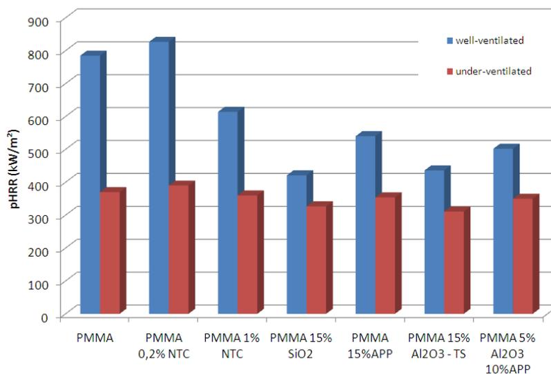
**Figure 4.** Comparison of pHRR for the test samples.
