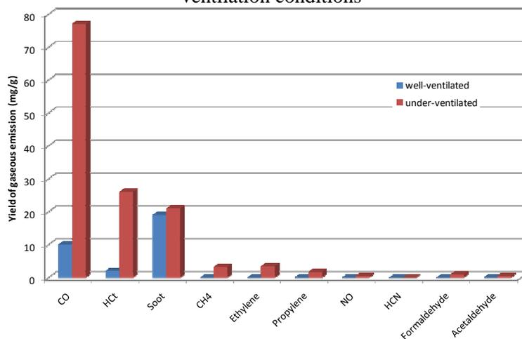
**Figure 8.** Emission yields of various gases from combustion of PMMA - 15 SiO2 in controlled-ventilation conditions
