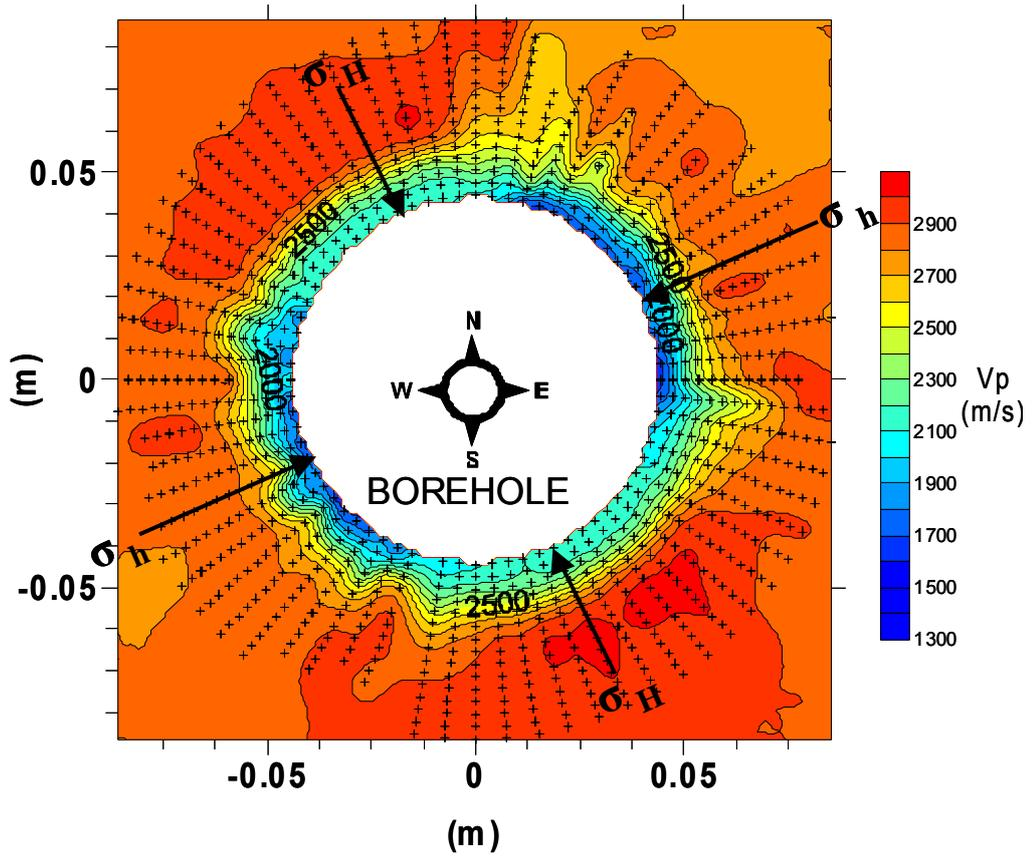
Figure 16: Image of the inversed velocity field.
