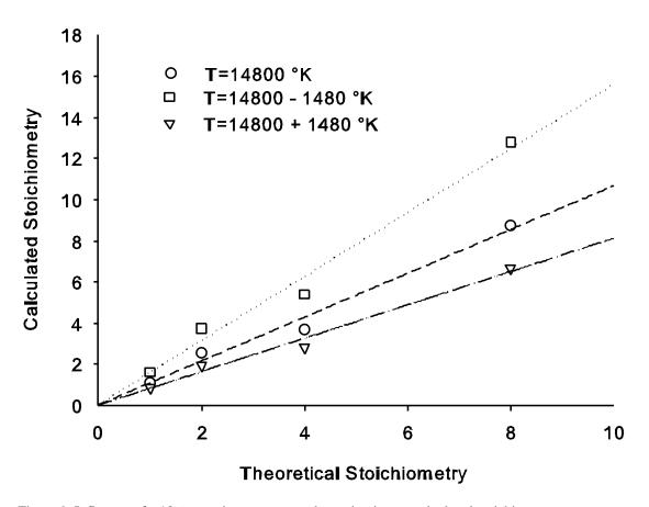
Figure 9. Influence of a 10% error in temperature determination on calculated stoichiometry.
