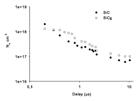
Figure 5. Temporal evolution of the electronic density during vaporization of SiC and  $SiC_8$  nanoparticles within the laser-induced plasma generated in the argon background gas.
