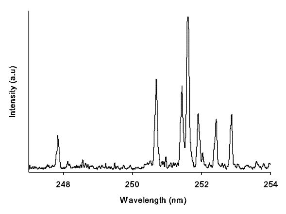
Figure 3. Spectrum recorded during vaporization of  $SiC_2$  nanoparticles within the laser-induced plasma (time delay of 4.2  $\mu$ s and an ICCD gate width of 2  $\mu$ s). The line on the left is C I at 247.86 nm. The six other lines correspond to Si I at, from left to right: 250.69 nm, 251.43 nm, 251.61 nm, 251.92 nm, 252.41 nm and 252.85 nm.
