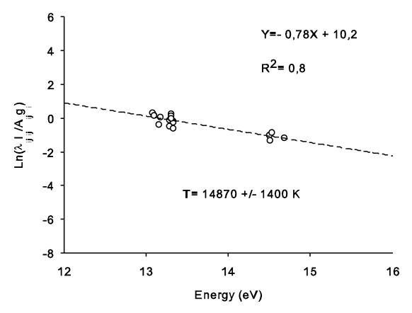
Figure 6. Example of Boltzmann plot obtained using argon lines (spectra recorded for time delay of 4.2  $\mu s$  and gate width of  $2\mu s$ ) during  $SiC_2$  Nanoparticle vaporization by the laser-induced plasma generated in the argon background gas.
