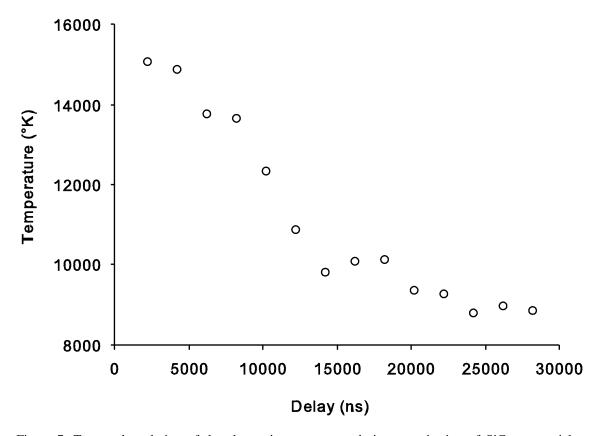
Figure 7. Temporal evolution of the electronic temperature during vaporization of SiC nanoparticles within the laser-induced plasma generated in the argon background gas.
