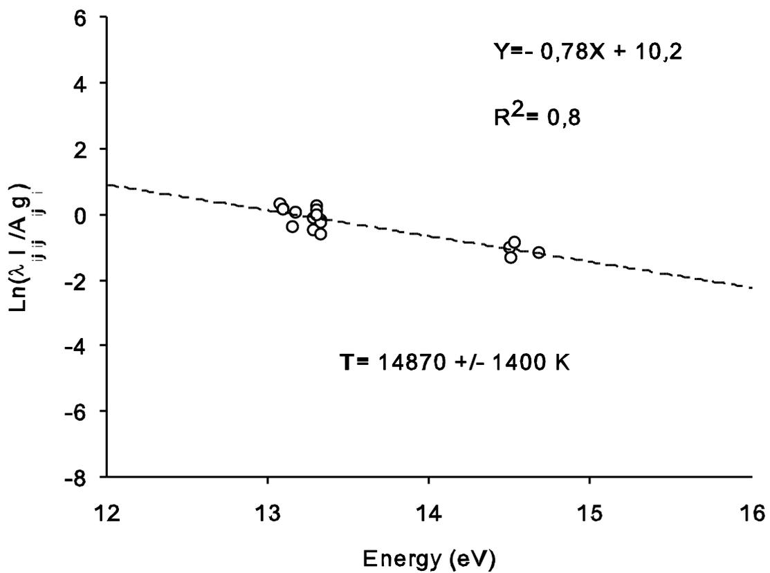
Figure 6. Example of Boltzmann plot obtained using argon lines (spectra recorded for time delay of 4.2  $\mu$ s and gate width of 2 $\mu$ s) during SiC<sub>2</sub> Nanoparticle vaporization by the laser-induced plasma generated in the argon background gas.
