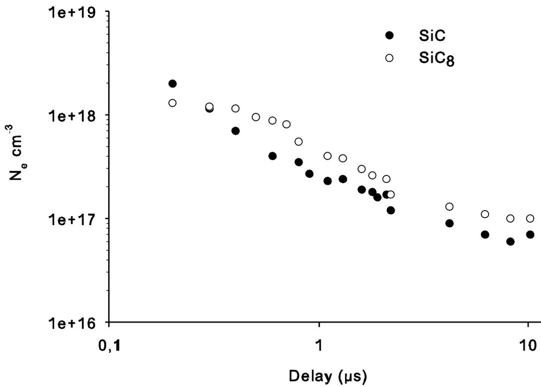
Figure 5. Temporal evolution of the electronic density during vaporization of SiC and SiC<sub>8</sub> nanoparticles within the laser-induced plasma generated in the argon background gas.
