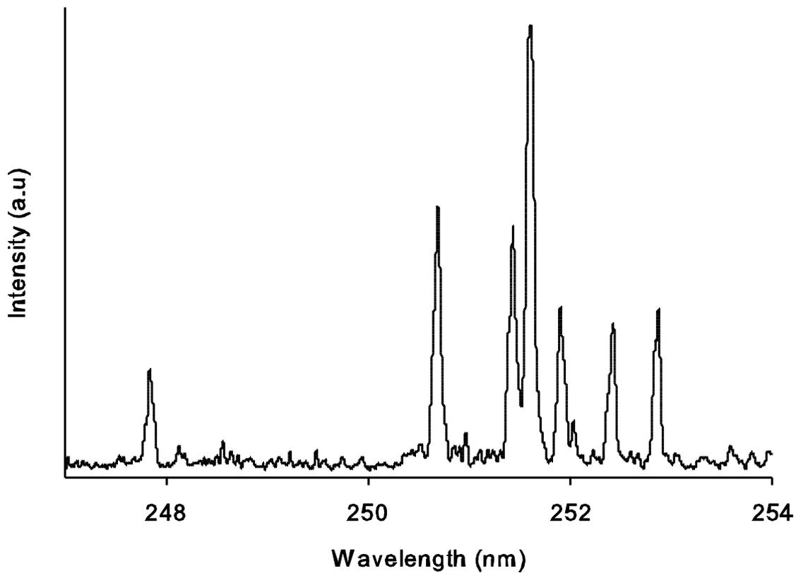
Figure 3. Spectrum recorded during vaporization of SiC<sub>2</sub> nanoparticles within the laser-induced plasma (time delay of 4.2  $\mu$ s and an ICCD gate width of 2  $\mu$ s). The line on the left is C I at 247.86 nm. The six other lines correspond to Si I at, from left to right: 250.69 nm, 251.43 nm, 251.61 nm, 251.92 nm, 252.41 nm and 252.85 nm.
