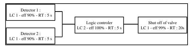
Figure 12: Architecture of safety function (LC1 - eff. 90% - RT: 30s)
