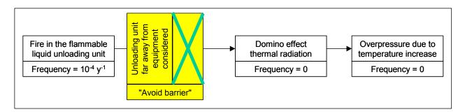
Figure 3: "Avoid" barrier in the fault tree
