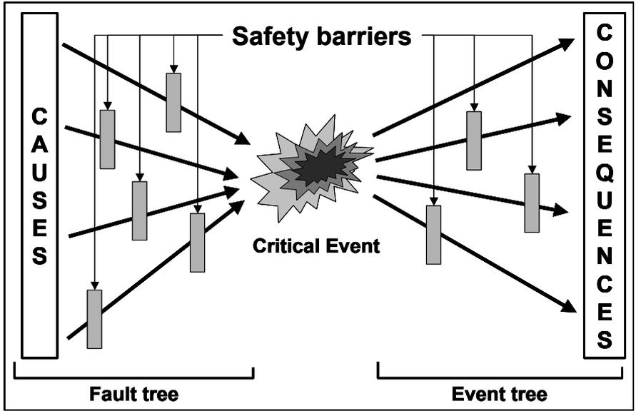
Figure 2: Complete bow-tie with identification of prevention or mitigation safety functions
