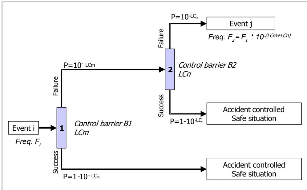
Figure 6: "Control" barriers – influence on the calculation of frequencies of events in term of level of confidence
