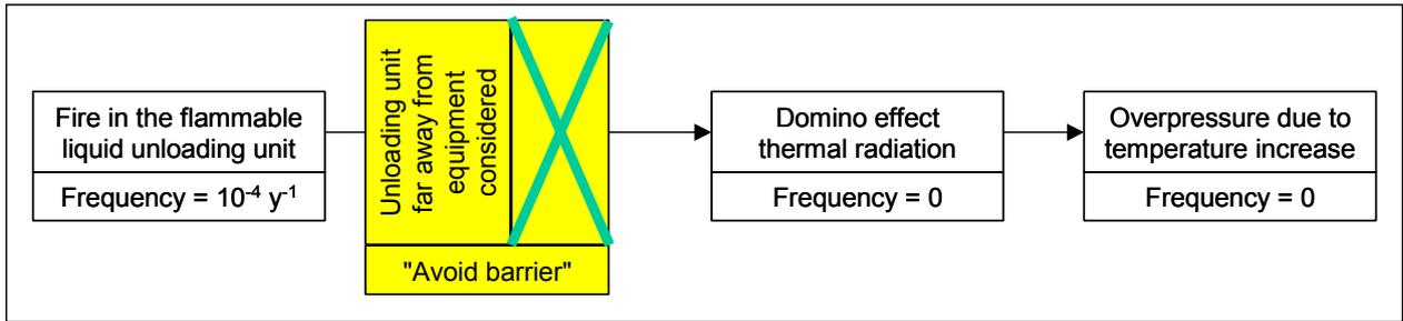
Figure 3: "Avoid" barrier in the fault tree
