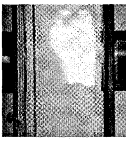
Figure 4 : Ignition of a starch dust air mixture by a CW-MM-Nd-YAG laser beam
