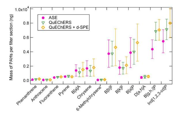
**Fig. 5.** Comparison of the average quantity of PAH per filter determined according to the used extraction procedure: ASE, QuEChERS and QuEChERS + d-SPE clean-up. Filter sections (1.5 cm²) originated from the same emission filter sample (n = 3). The error bars show the standard deviation of the triplicate analysis. \*6-Methylchrysene: surrogate standard (100 ng filter<sup>-1</sup>). Same analytical conditions as in Fig 3.
