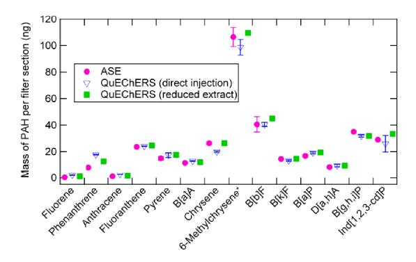
**Fig. A4.** Comparison of the average quantity of PAH per filter determined according to the used extraction procedure: ASE and QuEChERS. For QuEChERS, extraction solvent was acetonitrile (ACN). Filter sections originated from the same PM<sub>10</sub> ambient air filter sample (n = 3). The error bars show the standard deviation of the 10 (direct injection) or of the 3 (reduced extracts) essays. \*6-Methylchrysene: surrogate standard (100 ng filter<sup>-1</sup>).
