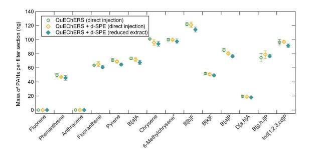
**Fig. A6.** Comparison of the average quantity of PAH per filter quantified according to the used extraction procedure: QuEChERS and QuEChERS + d-SPE clean up. Filter sections ( $\varnothing$  = 47 mm) originated from the same PM<sub>10</sub> ambient air filter sample (n = 3). The error bars show the standard deviation for the triplicate analysis. Extraction solvent was acetonitrile (ACN). \*6-Methylchrysene: surrogate standard (100 ng filter<sup>-1</sup>).
