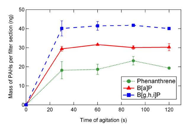
**Fig. 3.** Comparison of the average PAH quantity extracted for phenanthtrene, B[a]P and B[g,h,i]P according to the time of agitation in the QuEChERS procedure. Filter sections ( $\emptyset = 47$  mm) originated from the same PM<sub>10</sub> ambient air filter sample (n = 3). The error bars show the standard deviation for the triplicate analysis. Extraction solvent was acetonitrile (ACN) and the direct injection of the sample extracts was performed.
