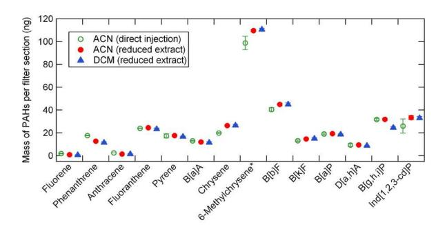
**Fig. 1.** Comparison of the average PAH quantity extracted according to the extraction solvent used (dichloromethane (DCM) or acetonitrile (ACN) - direct injection and injection of reduced extracts) with the QuEChERS procedure. Filter sections ( $\emptyset = 47$  mm) originated from the same PM<sub>10</sub> ambient air filter sample (n = 3). The error bars show the standard deviation for the triplicate analysis. \*6-Methylchrysene: surrogate standard (100 ng filter<sup>-1</sup>).
