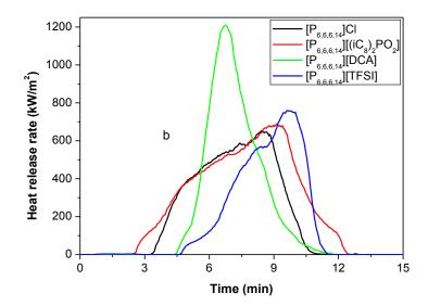
Figure 8: Comparison between total heat release from PCFC and FPA calorimeter
