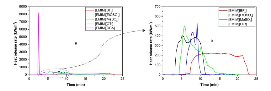
Figure 7: Combustion heat flux as a function of time during the combustion of PBILs
