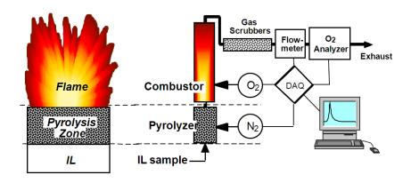
Figure 3: Schematic view of the FPA calorimeter system and instrument picture
