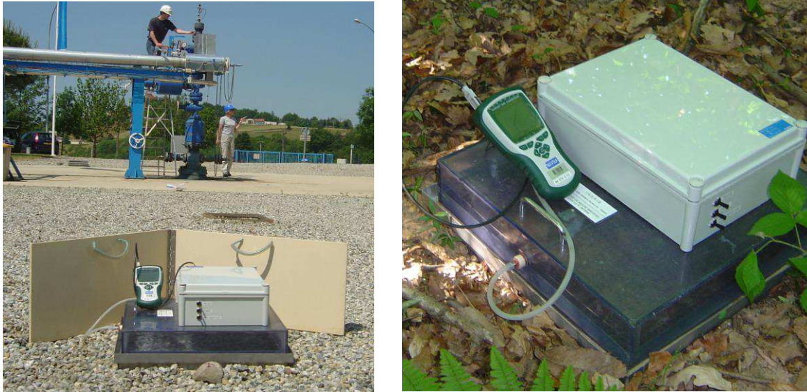
Figure 7. Device for CO 2 flux measurements at the ground/atmosphere interface
