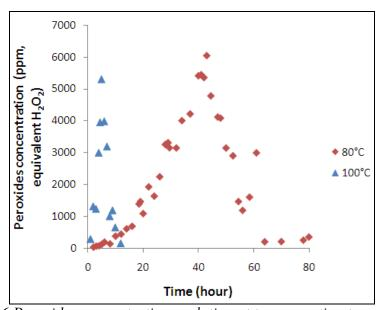
Figure 6.Peroxides concentration evolution at two operating temperatures
