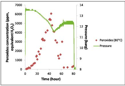
Figure 7.Peroxides concentration and pressure evolution at 80°C
