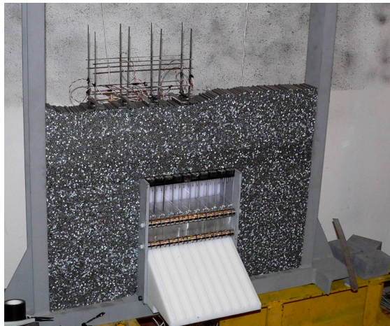
Figure 1. View of the small-scale experimental model (apparatus for the creation of the cavity at the centred bottom, Schneebeli material, building model on the ground surface).
